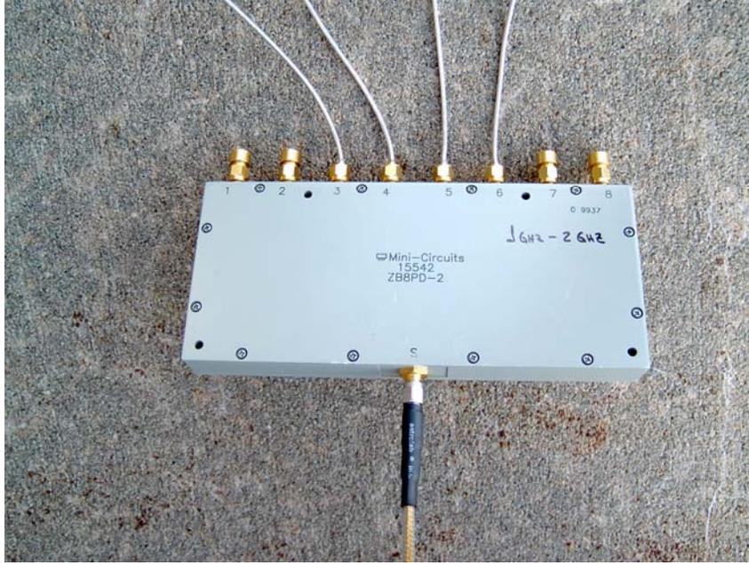
Figure 26: Mini-Circuits ZB8PD-2 power combiner used at 1350 MHz.
