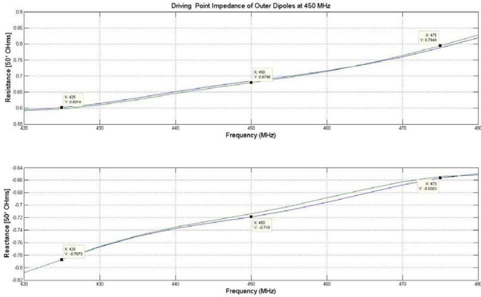
Figure 17: Driving point impedance of outer dipoles at 450 MHz (1 & 4)
