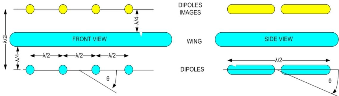
Figure 4: Front and side views of the dipole array composed of four true dipoles and images.
