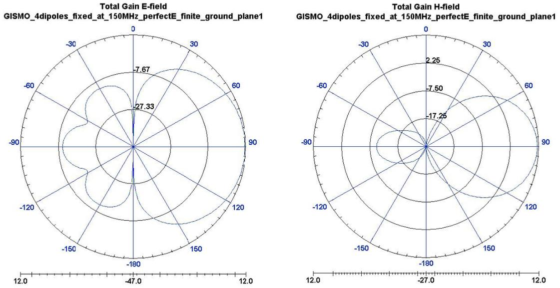
Figure 13: Antenna gain towards E-field (left) and H-field (right) at 150 MHz under a finite ground plane with weighting.
