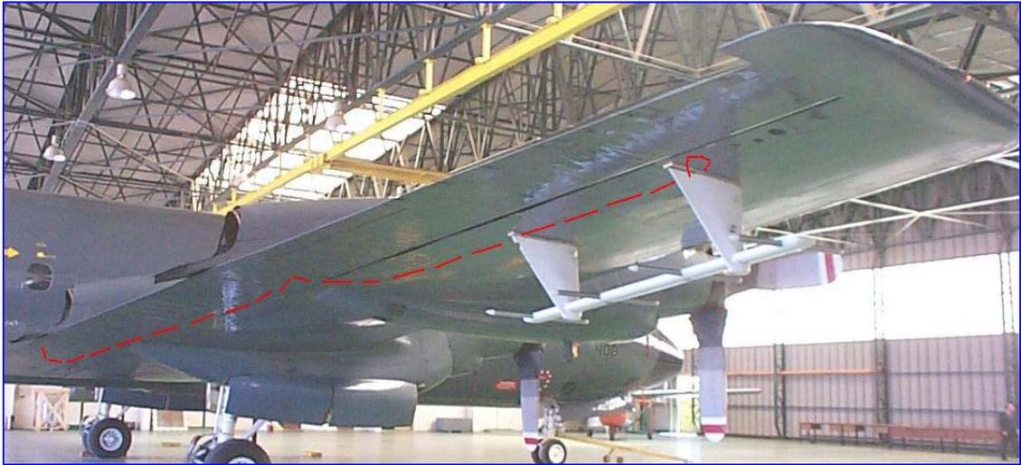
**Figure 2: Dipole antenna array mounting 2**
