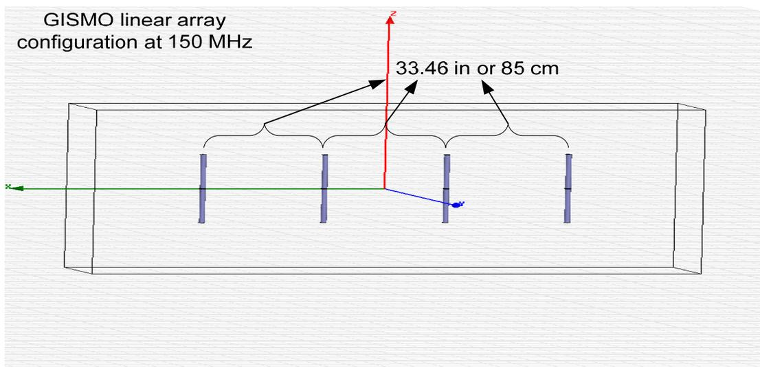
**Figure 8: GISMO antenna array configuration.**
