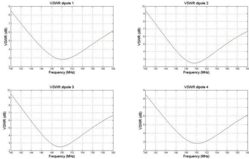
Figure 16: VSWR of each dipole at 150 MHz.
