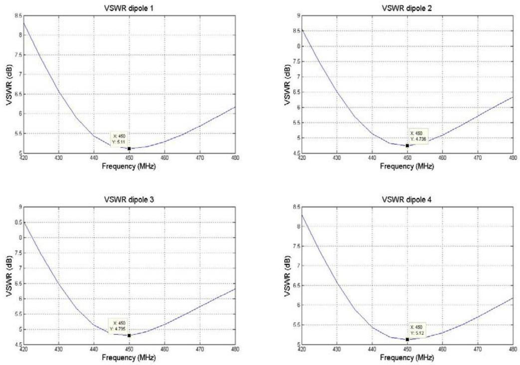
Figure 24: VSWR of each dipole at 450 MHz.
