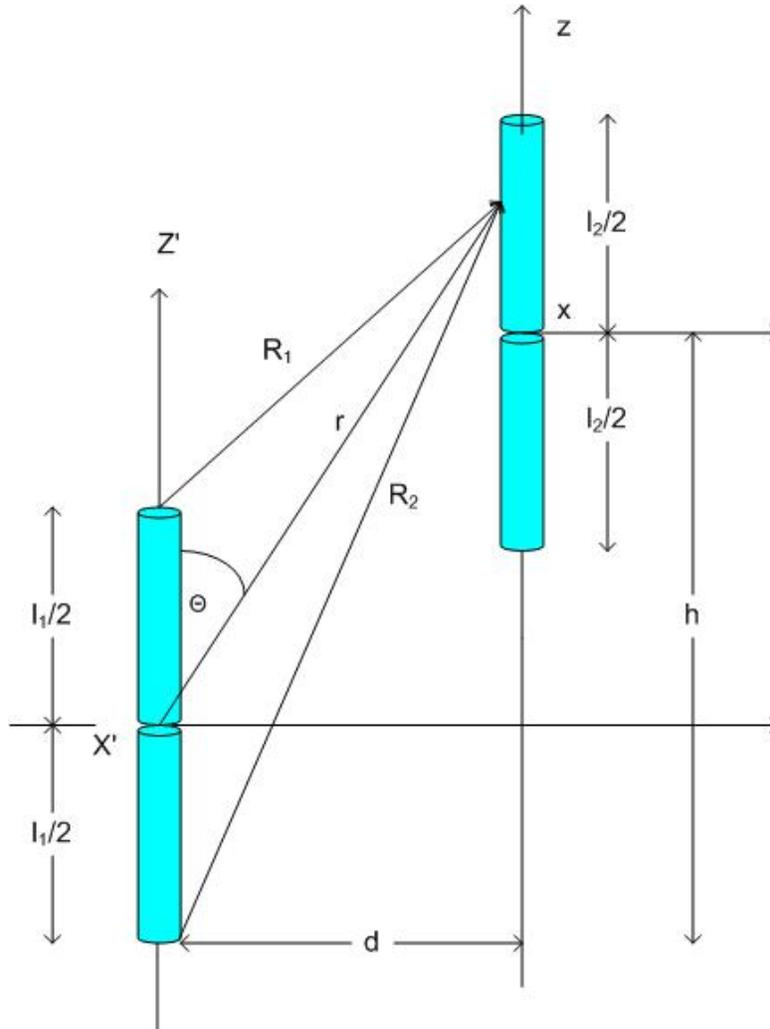
Figure 5: Dipole positioning for mutual coupling.
