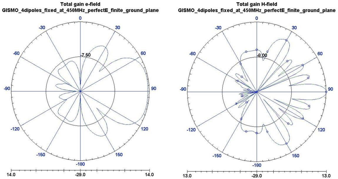
Figure 20: Antenna Total gain towards E-field (left) and H-field (right) at 450 MHz under a finite ground plane.
