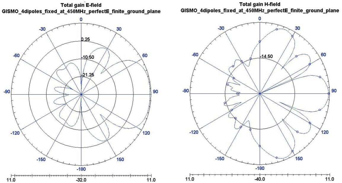
Figure 21: Antenna gain towards E-field (left) and H-field (right) at 450 MHz under a finite ground plane with weighting.
