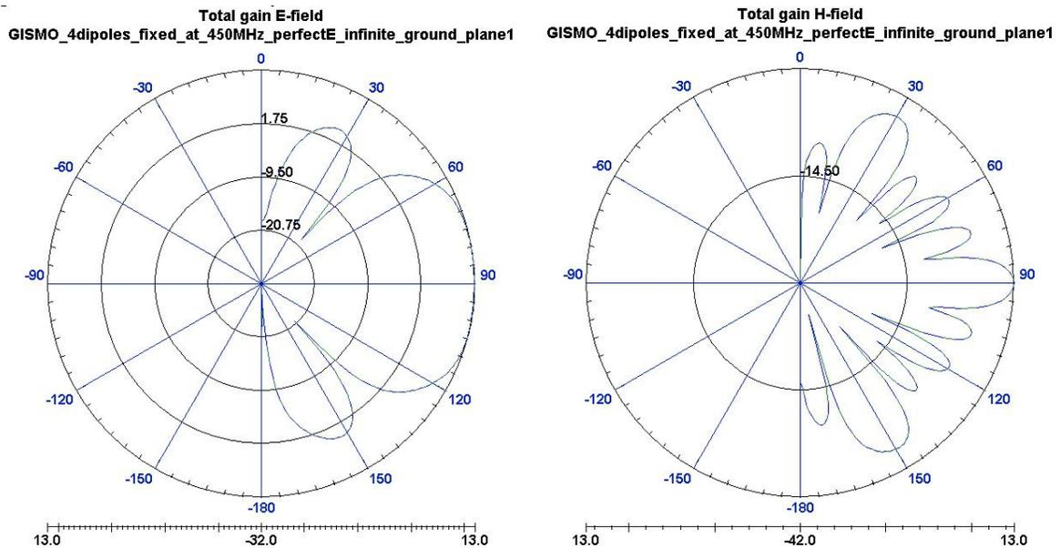
**Figure 19: Antenna Total gain towards E-field (left) and H-field (right) at 450 MHz under an infinite ground plane.**
