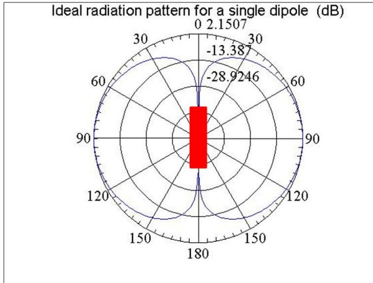
**Figure 3: Far-Field Radiation pattern for a single dipole.**
