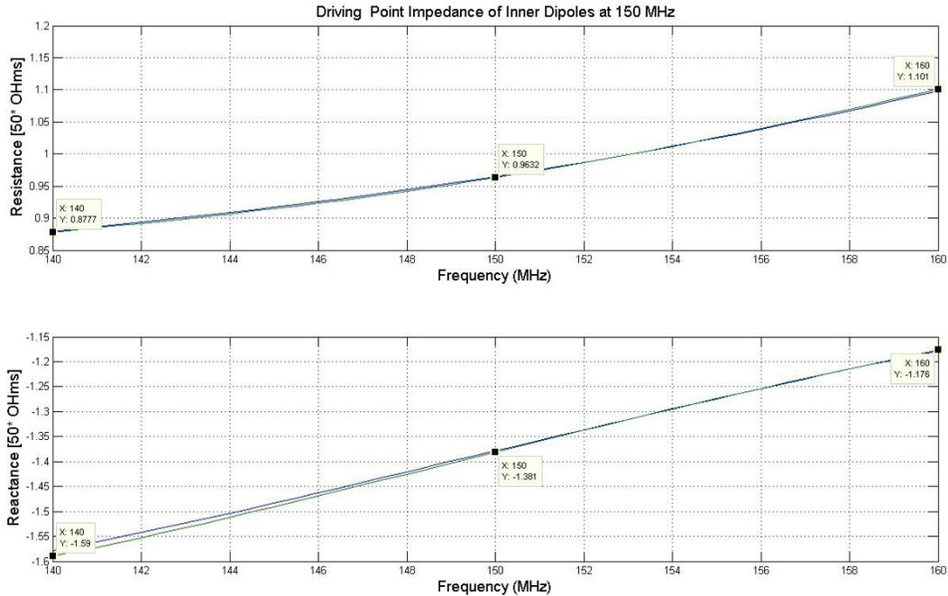
Figure 10: Driving point impedance of inner dipoles at 150MHz (2 & 3)
