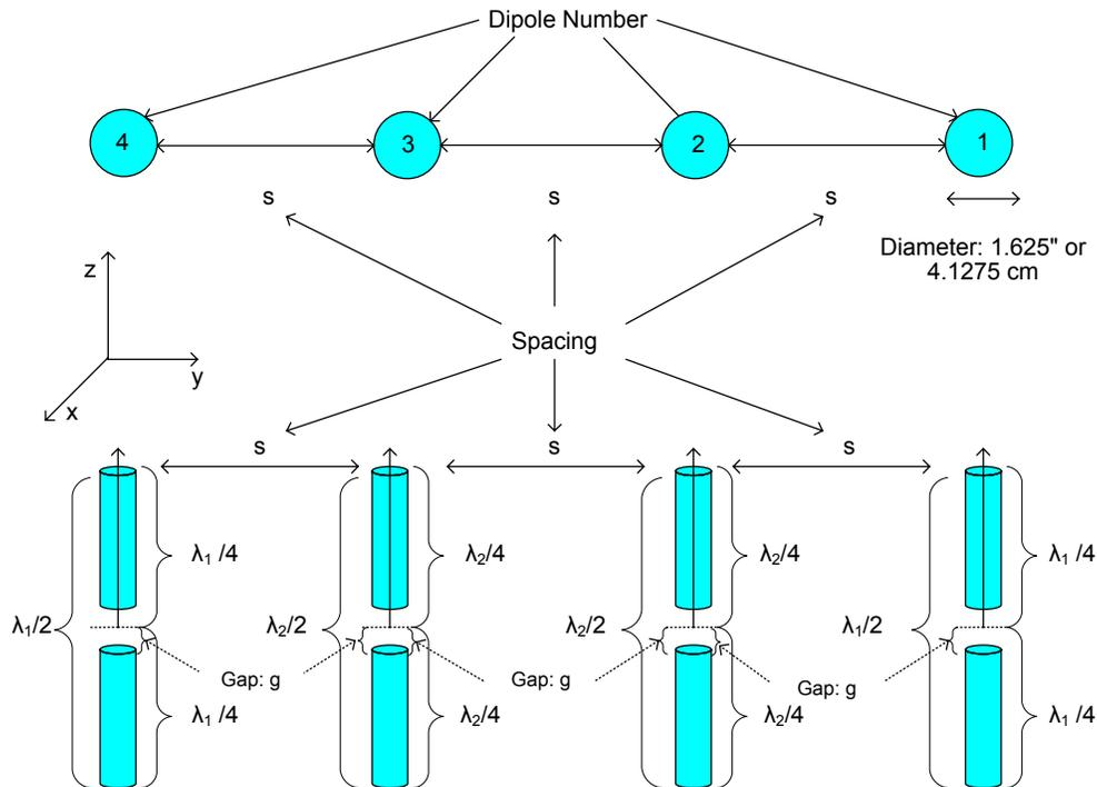
**Figure 6: Four-dipole antenna array at 150 [MHz]**
