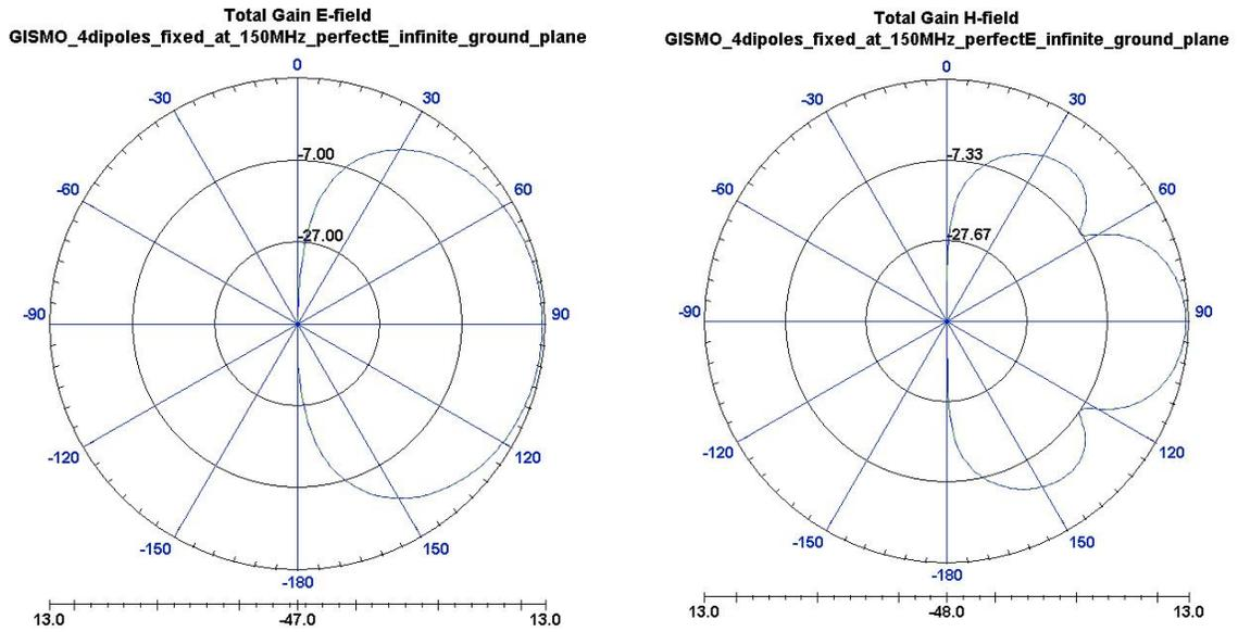
Figure 11: Antenna Total gain towards E- field (left) and H-field (right) at 150 MHz under an infinite ground plane.
