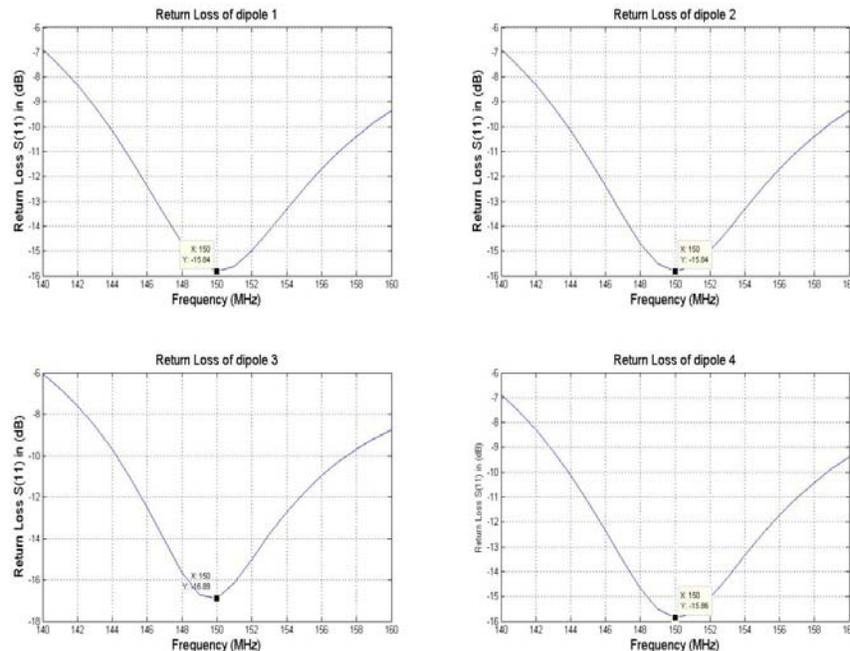
Figure 15: Return loss of each dipole at 150 MHz.
