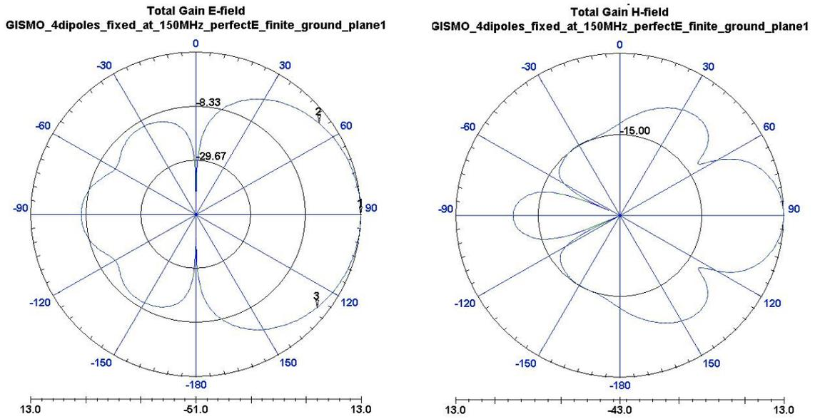
Figure 12: Antenna Total gain towards E- field (left) and H-field (right) at 150 MHz under a finite ground plane.
