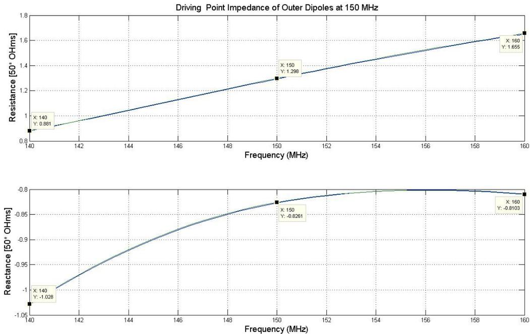
Figure 9: Driving point impedance of outer dipoles at 150 MHz (1 & 4)
