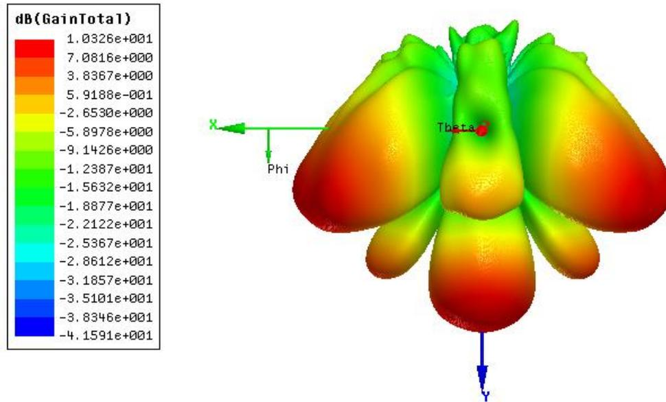
Figure 22: Antenna 3-D gain at 450 MHz under an infinite ground plane.
