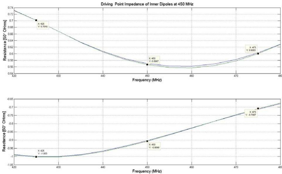
Figure 18: Driving point impedance of inner dipoles at 450 MHz (2 & 3)
