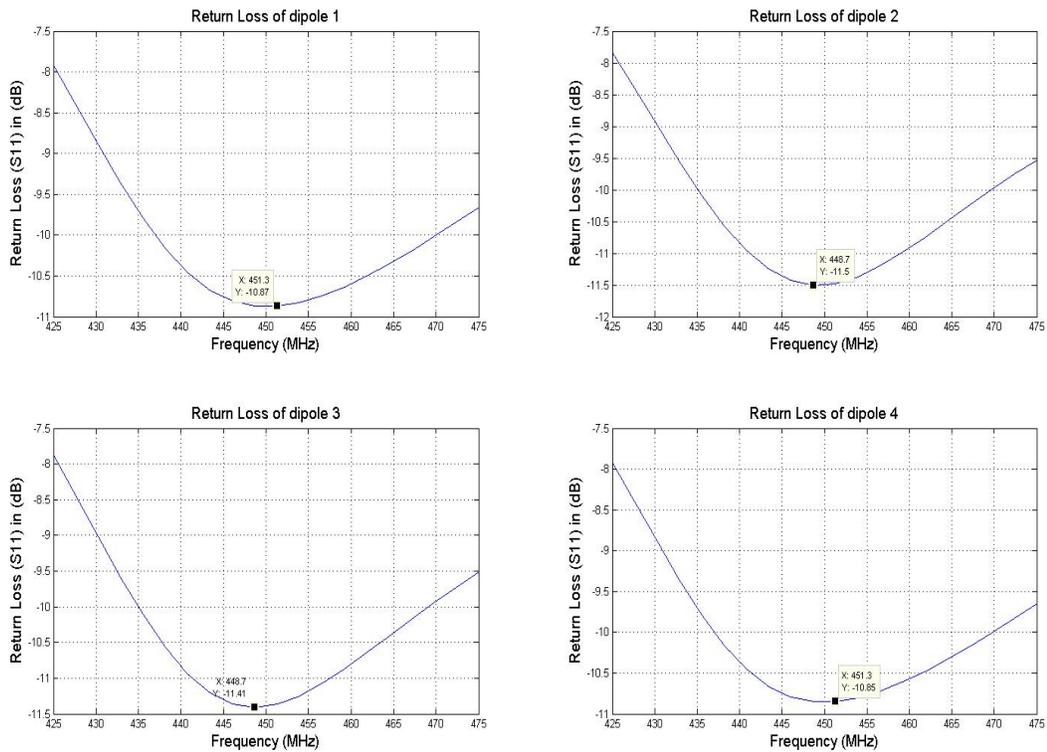
Figure 23: Return loss of each dipole at 450 MHz.
