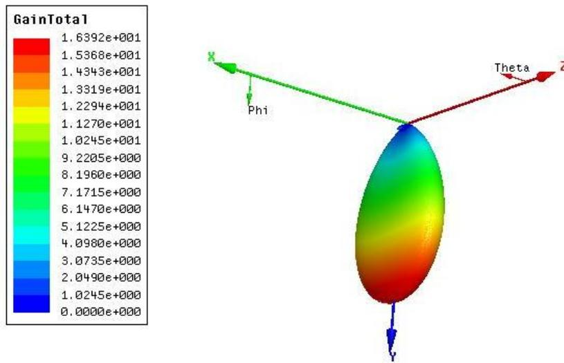
Figure 14: Antenna 3-D gain at 150 MHz under an infinite ground plane.
