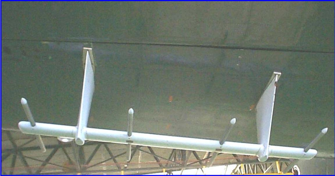
**Figure 1: Dipole antenna array mounting 1**
