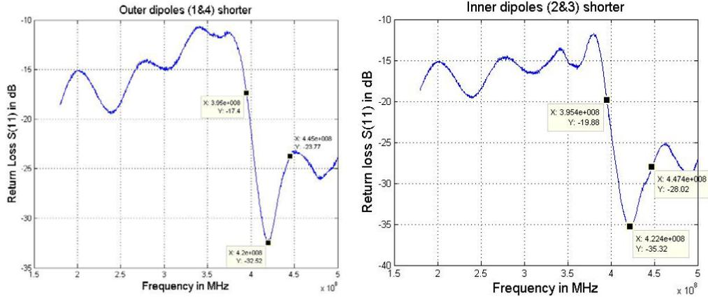
**Figure 27: Return loss of the array when outer dipoles are shorter (left), and when inner dipoles are shorter (right)**
