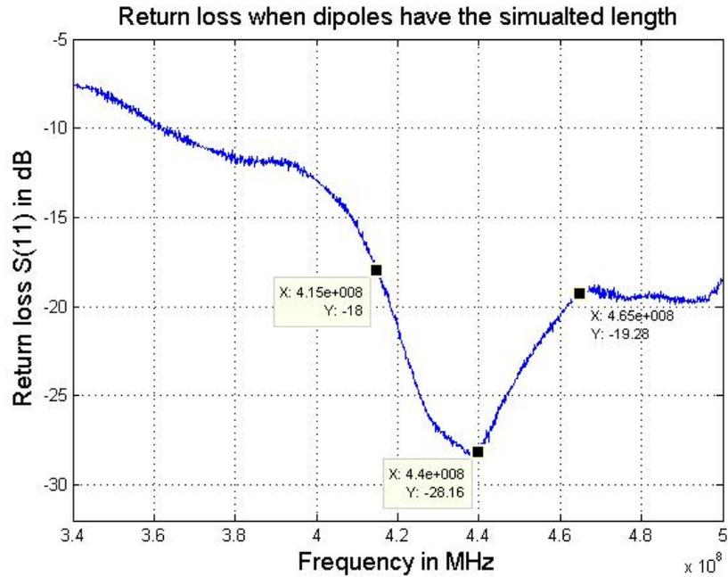
**Figure 28: Return loss of the array when dipoles have the simulated length.**
