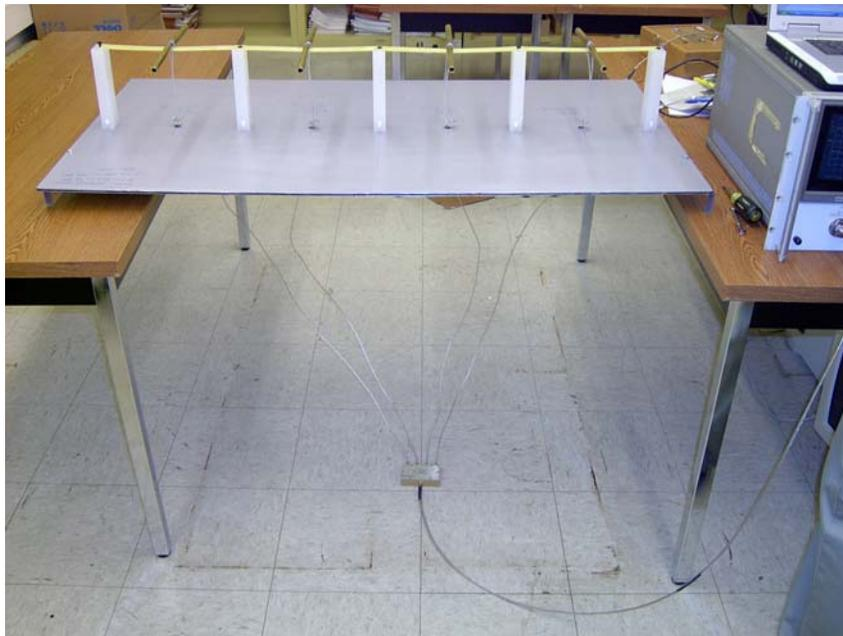
Figure 25: Mini-Circuits ZB4PD1-500 power combiner used at 450 MHz.
