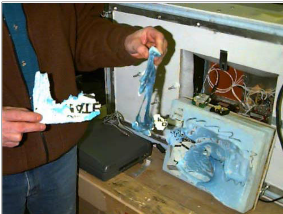
Figures 5&6. Example plot of RCS vs Orientation (Azimuth) Angle (above); melted South Pole transponder (below).
