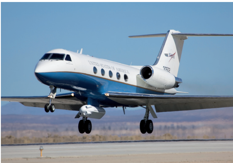
Figure 3: UAVSAR on the NASA Gulfstream G-III. NASA photo: Tom Tschida. ED07 0027 39.
