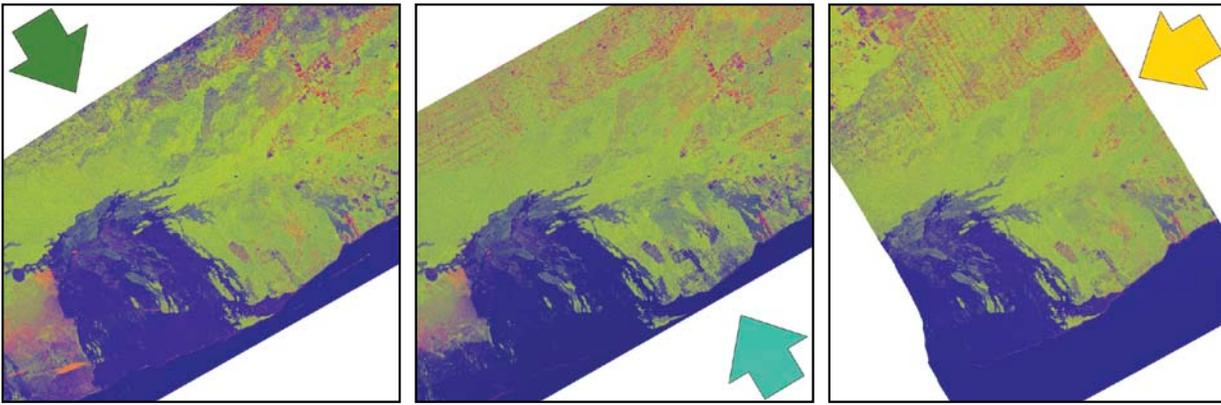
**Figure 4:** Color-coded VanZyl decompositions. The arrow indicates the radar look direction.
