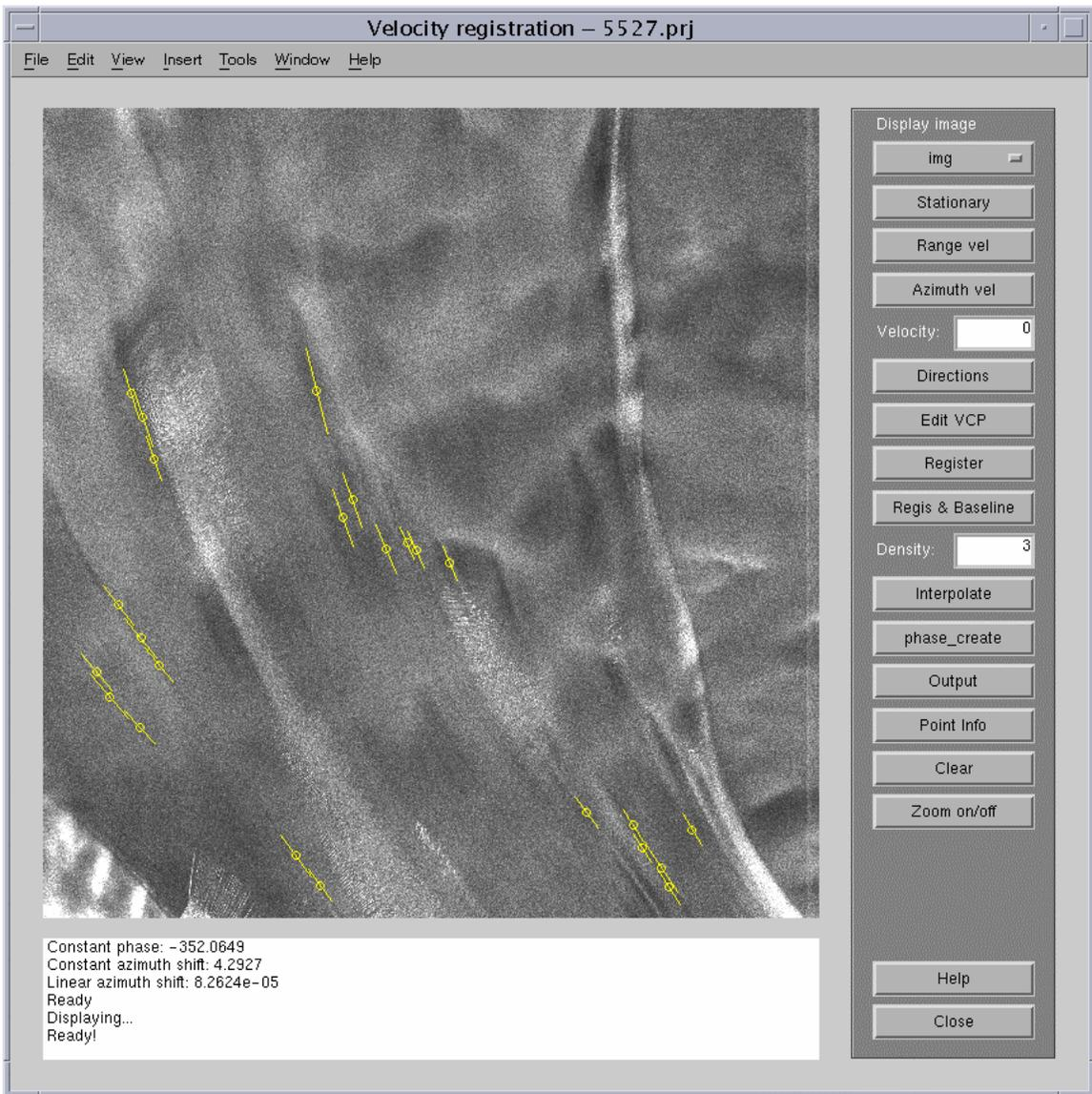
Figure 6.3: Flow direction control points are selected in velocity calibration
