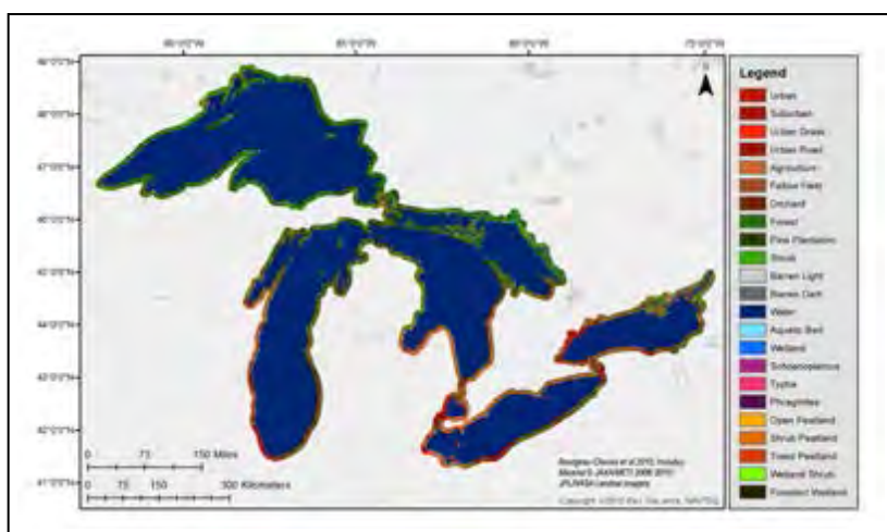
Figure 1. Land use land cover map of the coastal Great Lakes with a total accuracy of 94%. Click here for link to full map (http://geodjango.mtri.org/coastal-wetlands/). Bourgeau-Chavez et al. 2015. Includes Material © JAXA/METI 2008, 2010; JPL/NASA Landsat imagery.
