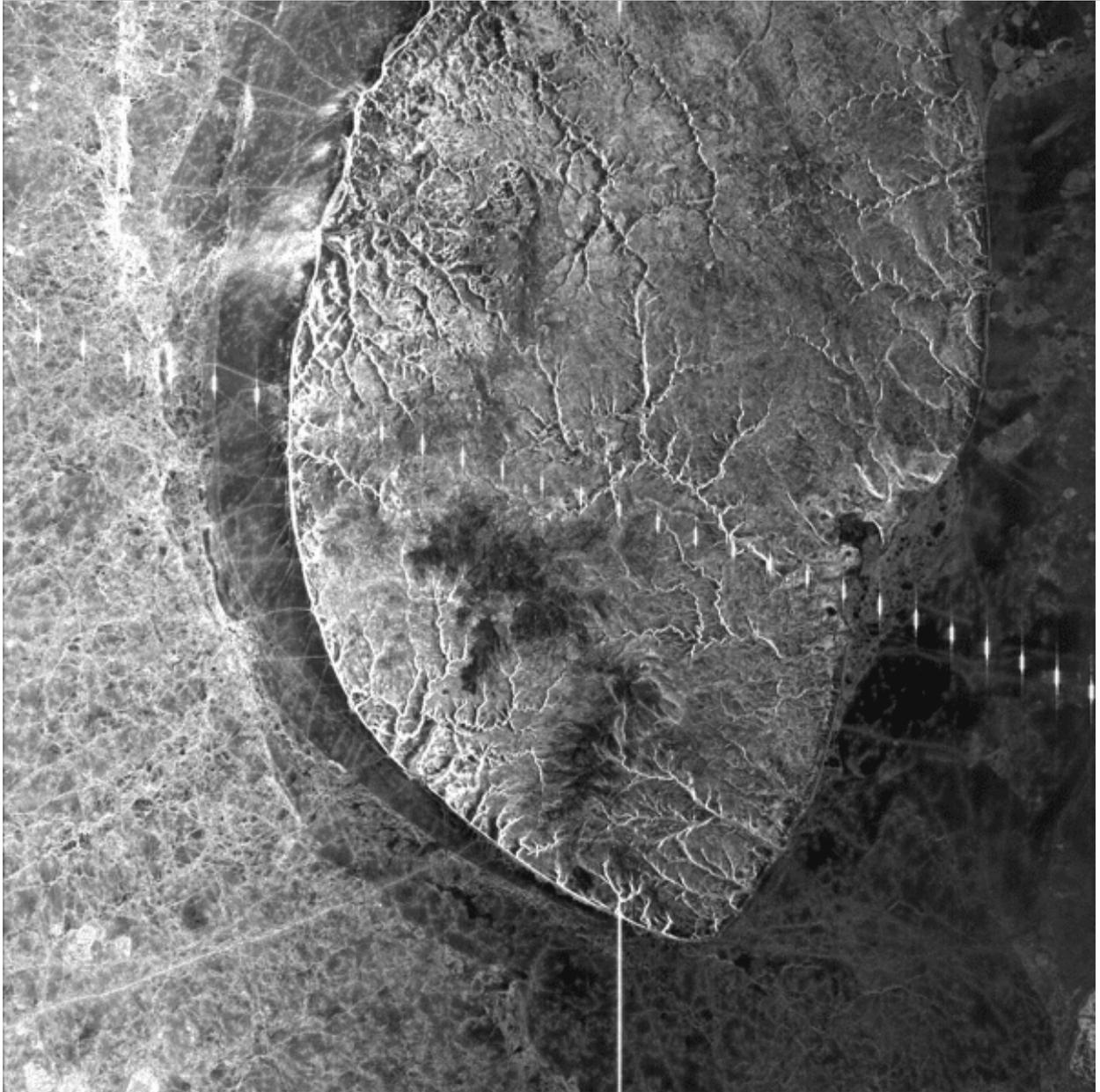
Dashes: The dash pattern across this image occurs in several Seasat images. It is noted that the whenever the dashes occur, the calibration pulse stops. This indicates that the dashes were intentionally placed into the signal data by Seasat engineers.
