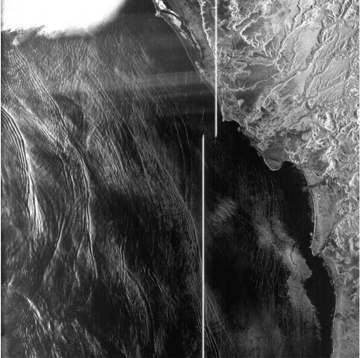
Non-regular Banding: It is common for across-track banding to show some curvature, as is displayed across the top of this image. This is due to the range migration portion of SAR focusing.
