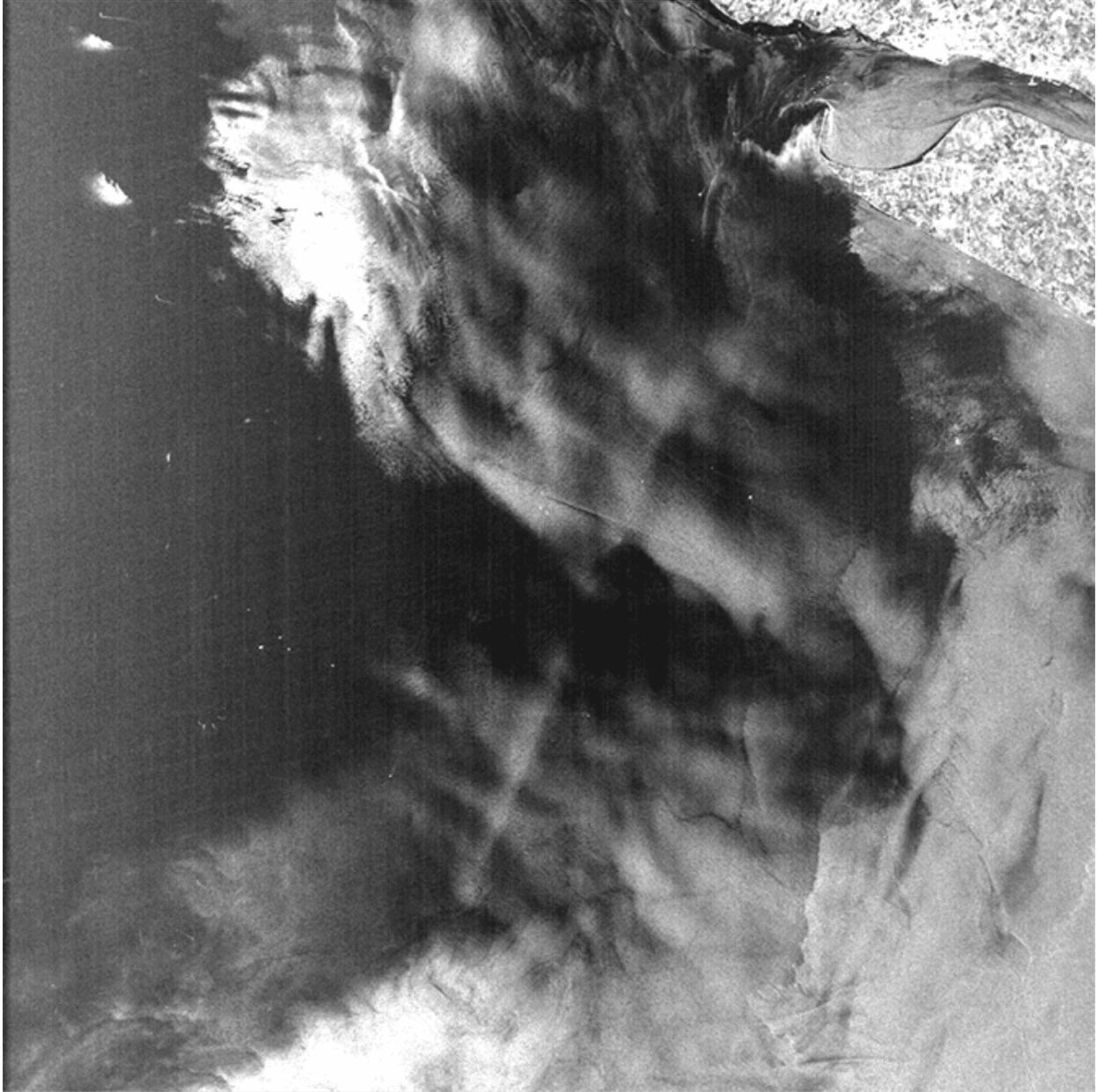
Along-Track and Across-Track Streaks: Some imagery evidences multiple data quality anomalies, like this image with both across-track and along-track streaks.
